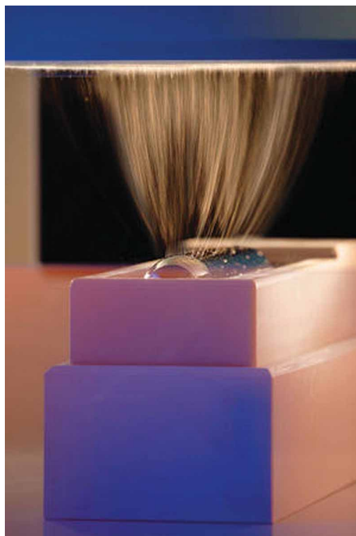
Figure 2. Rotating electrode 29 the essence of Nanospider Technology TM for making commercial nanofibers (reprinted with permission from Nanopeutics).
